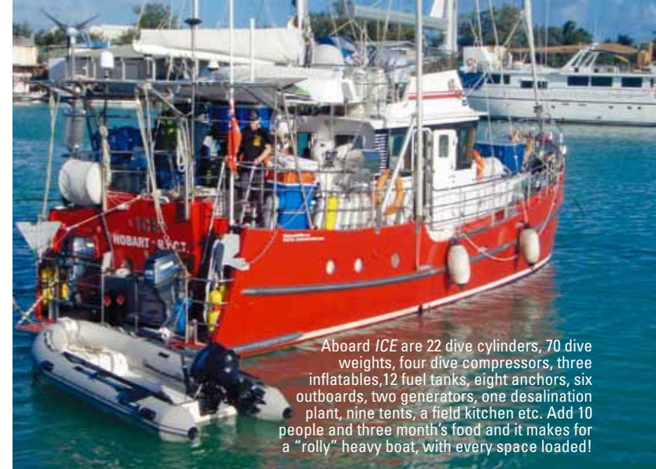
Aboard *ICE* are 22 dive cylinders, 70 dive weights, four dive compressors, three inflatables, 12 fuel tanks, eight anchors, six outboards, two generators, one desalination plant, nine tents, a field kitchen etc. Add 10 people and three month's food and it makes for a "rolly" heavy boat, with every space loaded!
