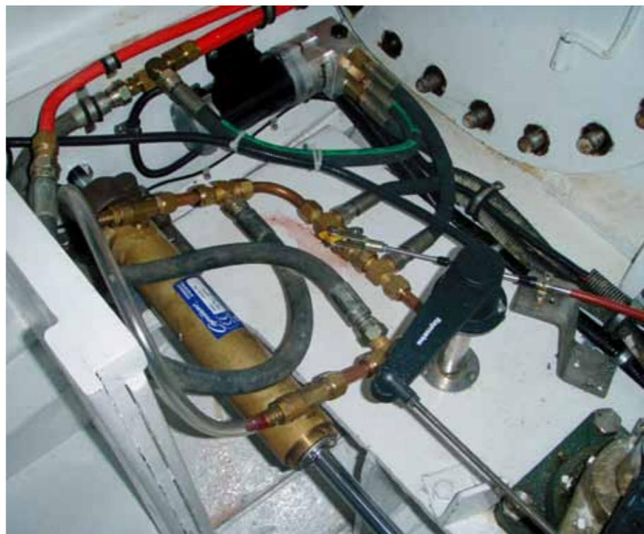
The starboard main steering ram has the backend of the shaft moving through a hole in the bulkhead. When the four mounting bolts released, the ram would lift and the rod rubbed making a bigger hole! This ram has a connected autopilot. My second independent portside ram is only connected to a second autopilot, acting as my first emergency steering if needed. I also have an emergency tiller setup.
