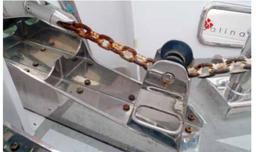
Above: Each year we lose 30cm of zinc galvanised chain due to corrosion by its connection to the stainless steel anchor and swivel.
