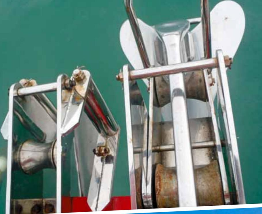
Left: My stainless steel 110lb anchor and port anchor chute with vertical rollers setup to take heavy side loads and not cut the rope – handy for groundings when you need to pull the boat sideways or if you set a second anchor at 60° to the original chain and anchor.
