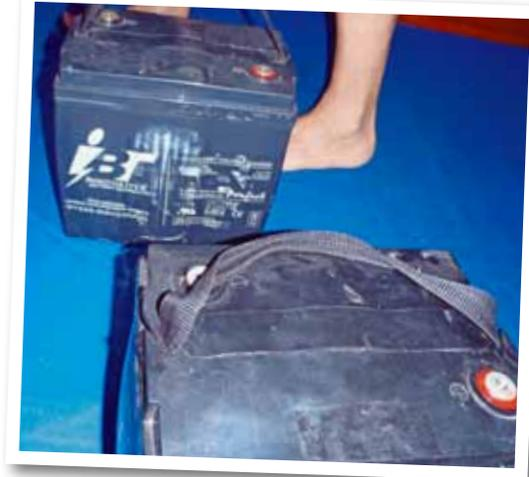
My fried 12V battery bank from last season, courtesy of a faulty DC/DC charger — they expanded and cracked but didn't explode!
