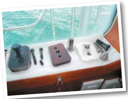
Bill's "Super Pusher" tool on the left, my "homemade" tool in the middle and the official "white" JD tool on the right... all useless! at pushing the seized injector pump shaft out of the gear.
